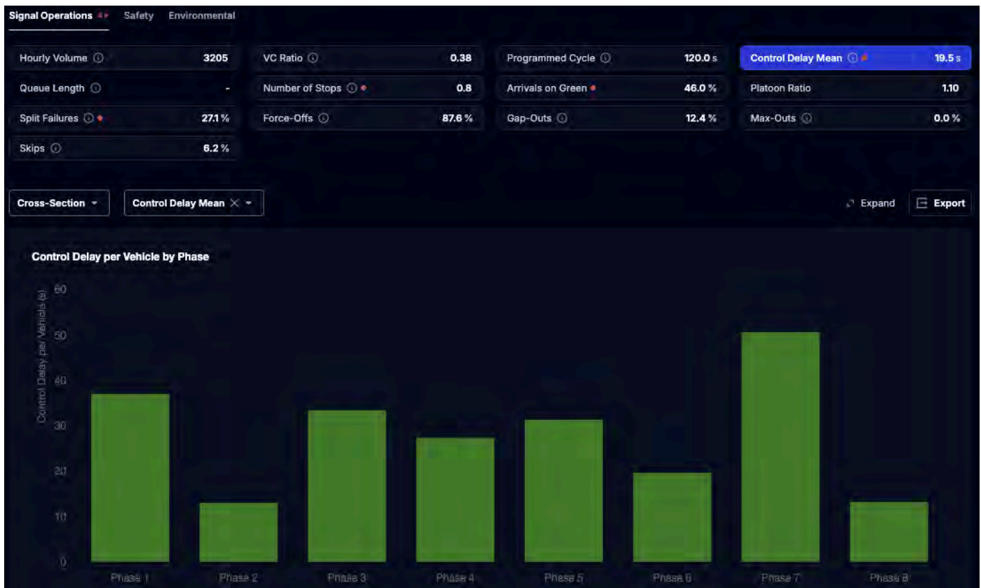
Figure 3 - Average Delay per Approach per Intersection. Flow Labs provides Average Delay and Median Delay per approach per intersection. This can be visualized via the cross-sectional chart (shown above) or on a time series or time of day chart. Users can also click into these individual phases to get a detailed diagnostic of LOS and delay on a per vehicle basis.
