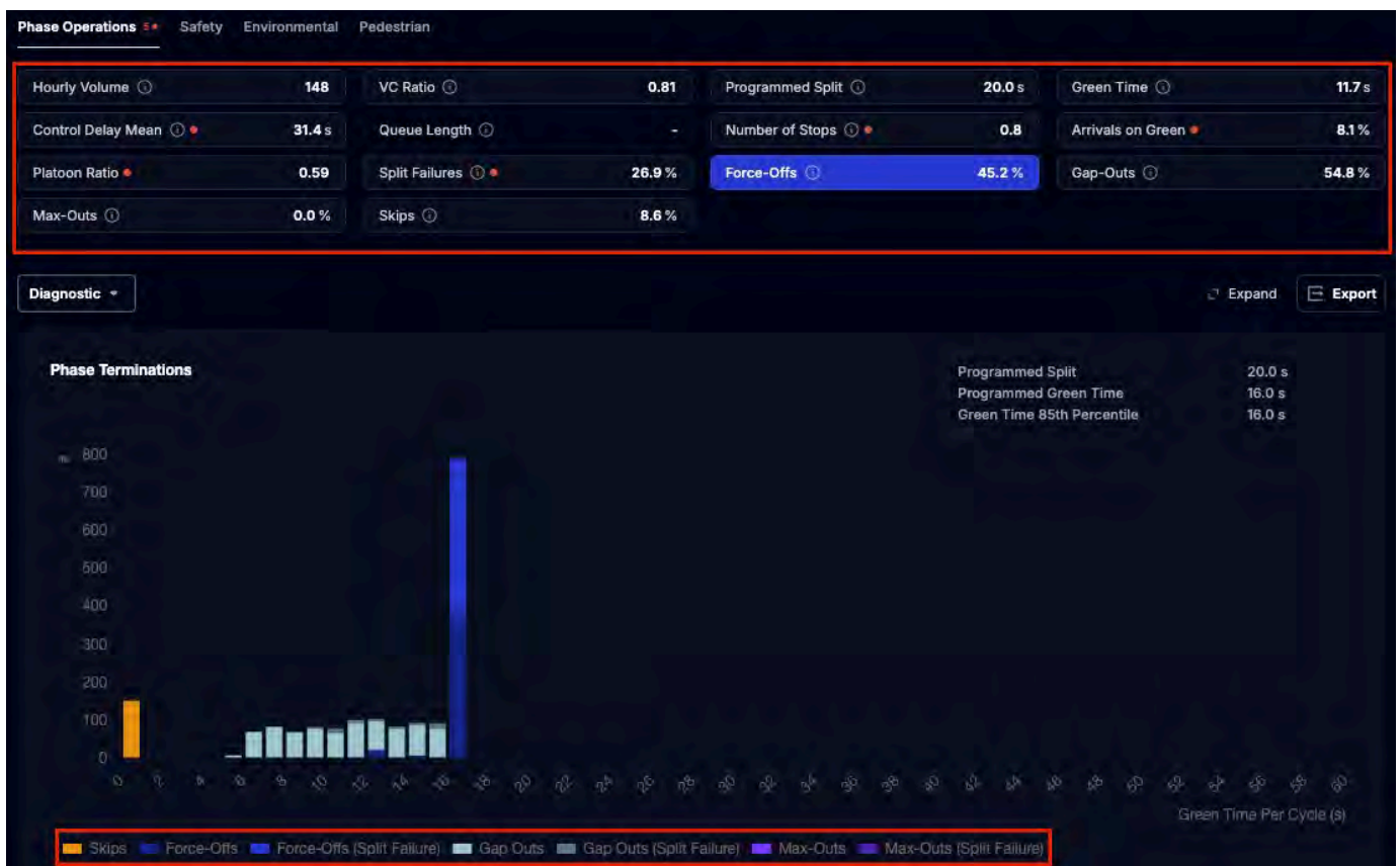
Figure 2 - Standard ATSPMs. As defined in Flow Labs Performance Measures appendix, ISPMs offer all the standard Purdue ATSPMs, including Gap-Outs, Max-Outs, Force-Offs, and Skips. Flow Labs provides diagnostic, time of day, and time series charts for each metric.
