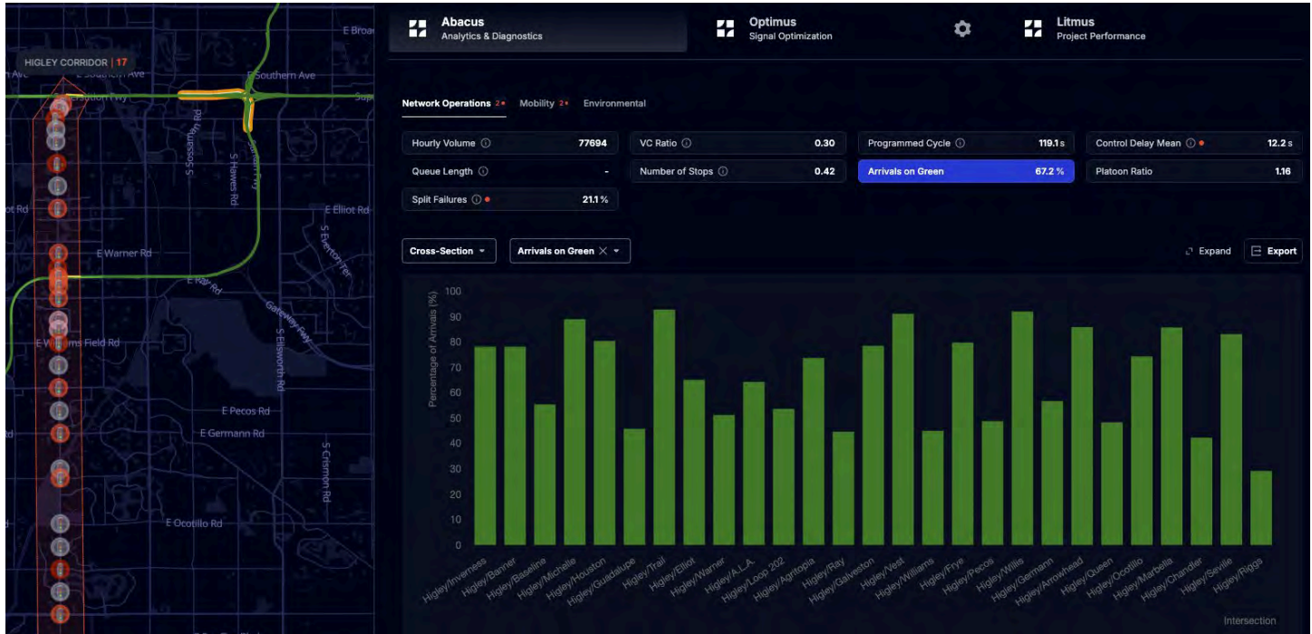
Figure 7 - Corridor Operations and AOG. Easily evaluate corridor operations and performance using a number of performance metrics including AOG. Luminus Plus visualizes these metrics using cross-section charts to easily see where AOG is the highest or lowest or if there are any outliers.
