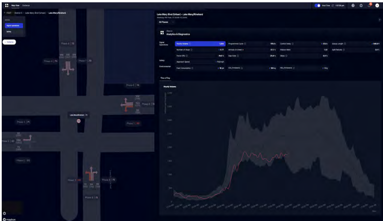
Figure 1 - Intersection Demand. Collect vehicle turning movement counts, corridor volumes, and speed data with sub-1 minute latency and no additional infrastructure. Explore diagnostic histograms, time series charts, and TOD visuals to better understand why issues occur. Immediately identify non-recurring congestion, major queues, and incidents and alert/notify instantly when issues arise.
