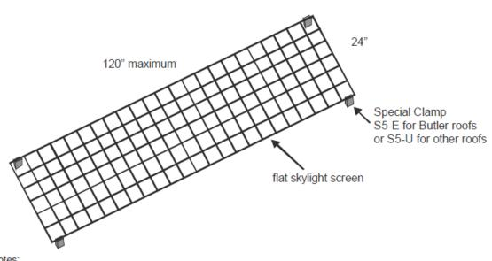
This is a custom, low profile skylight screen for a standing seam roof. Special clamps are provided to attach screen to the standing seam with no roof membrane penetration
