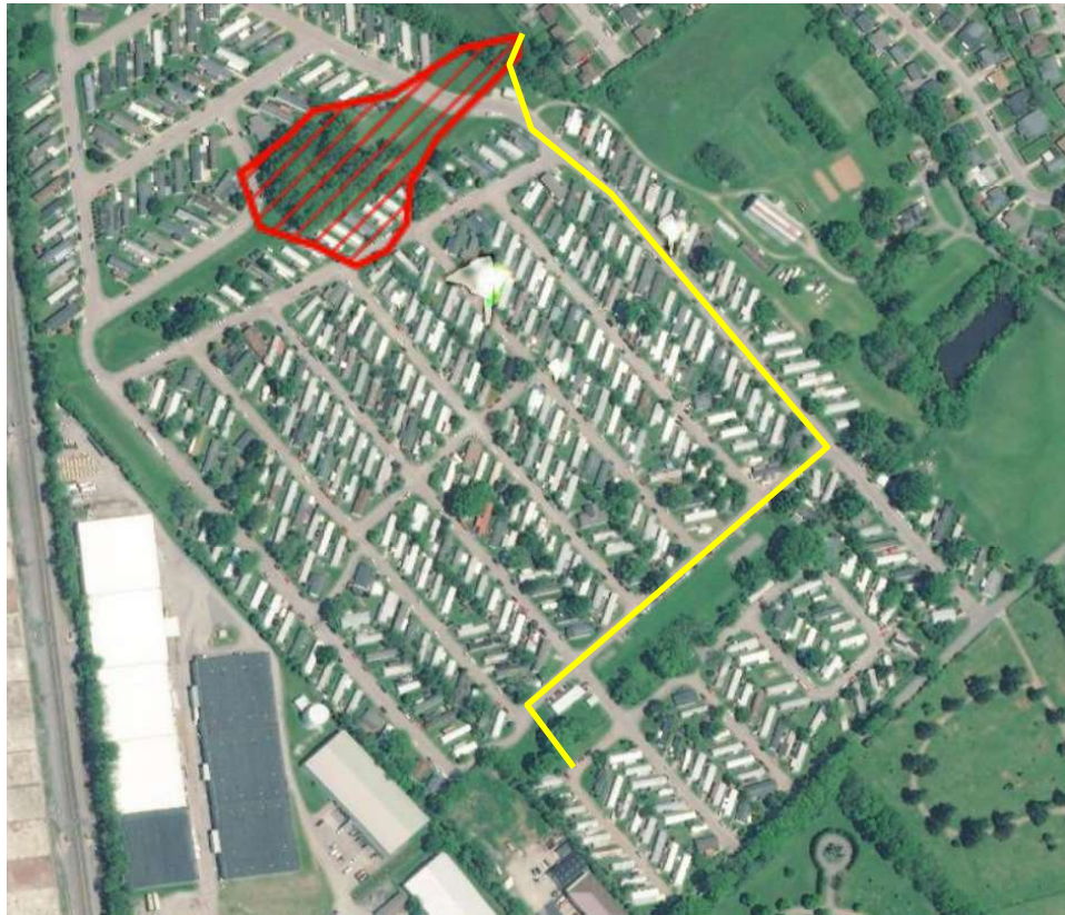
Figure 2: The KGS mapping indicated a sinkhole (red outline) is located near the north end of the proposed alignment (yellow line).
