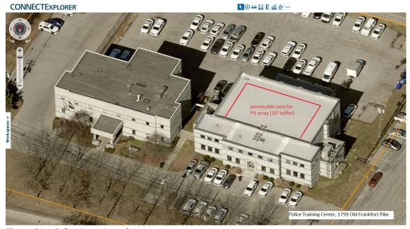
Figure 01 – Solar Array Location
