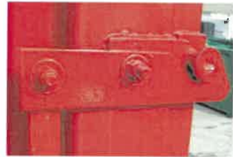
Optional ratchet-style rear door closing device secures the container.
