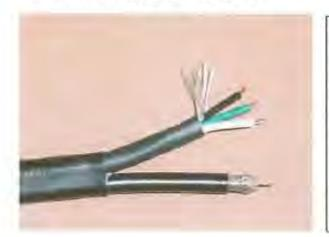
This is a picture of the ISOTEC Siamese cable. It is recommended that the outer cable jacket be cut away completely on the drip loop portion, to reduce strain on the camera BNC and Deutsch connectors. A suitable waterproofing compound should also be used to seal the "Y" junction were the video and power cable exit the outer jacket. This will help to prevent water from wicking down the cable and accumulating inside.
