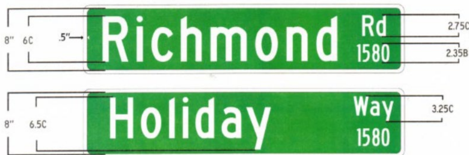
Figure 2-2: Nine (9) inch enhanced street name signs for public streets
