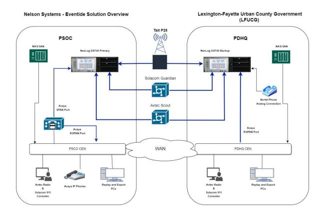
Each NexLog740DX will be deployed in a redundant fashion, with a primary and secondary. Eventide assumes the primary and secondary NexLog740DX will be in geodiverse locations for added resilience and disaster risk mitigation.
