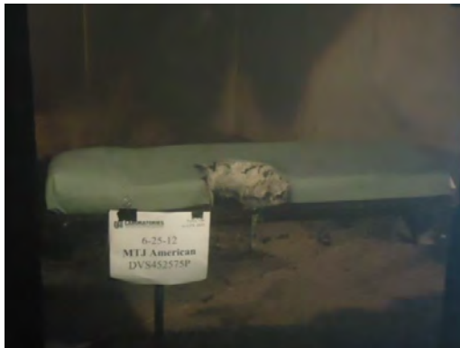
PHOTO 3. Mattress After Testing to 16 CFR 1633
