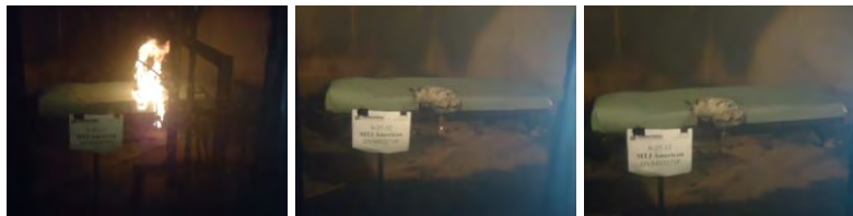
PHOTO(s) 2. Mattress During Testing to 16 CFR 1633
