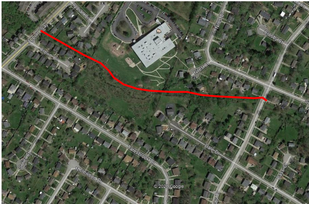
Figure 3: Proposed alignment from Appian Way to Cosby Drive. This section is about 1,650 linear feet with two road crossings (Appian Way and Crosby Drive).
