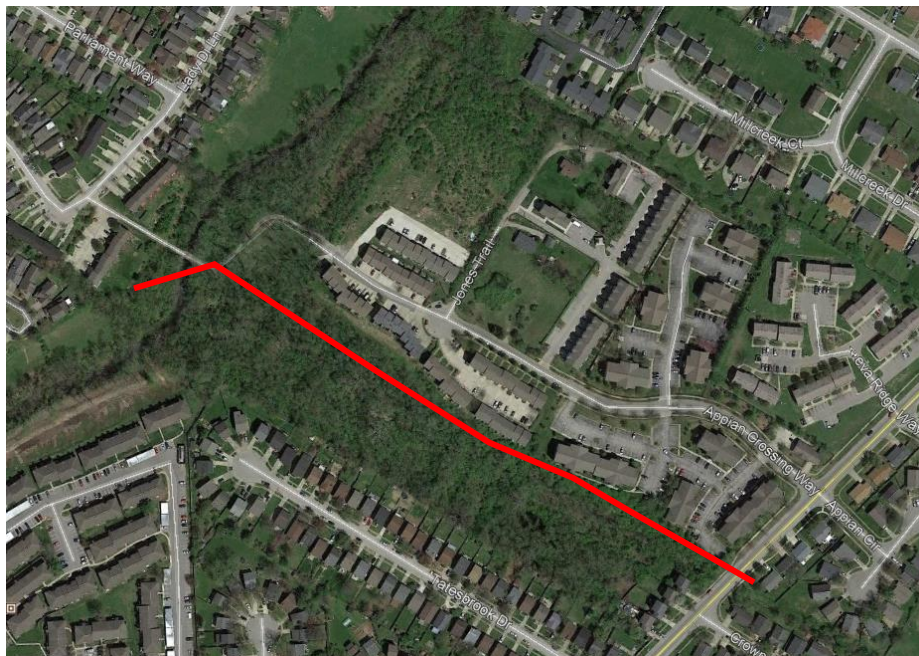
Figure 2: Proposed alignment of the proposed sewer line from West Hickman Creek to Appian Way. The length is about 1,700 feet.
