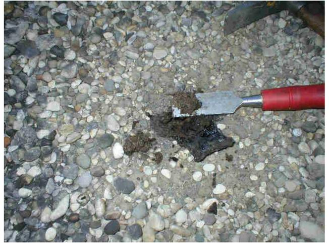
B) Area #2 Core Cut -Saturated Perlite Insulation
