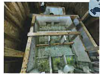
A physical model provides detailed insights to improve operations and mitigate troublesome pump intakes.
