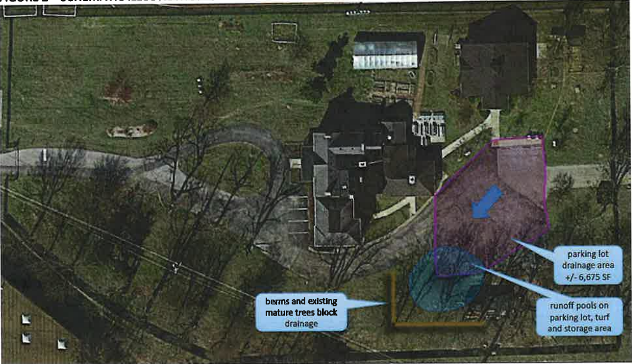
FIGURE 2 – SCHEMATIC ILLUSTRATION OF EXISTING CONDITIONS AT 519 WEST 4 TH STREET (FROM APPLICATION)
