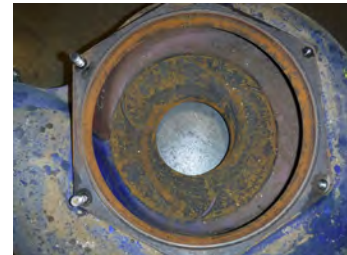
Inspection photo showing pitting on the existing dry weather pump impeller likely caused by vortices.
