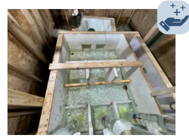
A physical model provides detailed insights to improve operations and mitigate troublesome pump intakes.
