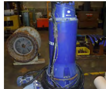
Pulled existing damaged dry weather pump.
