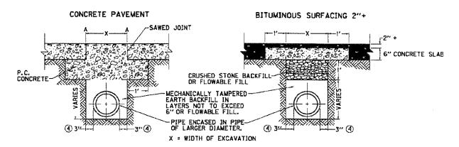
REPLACE CONCRETE PAVEMENT WITH NEW PAVEMENT SAME THICKNESS OF EXISTING PAVEMENT.
