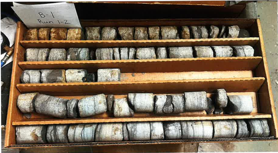
Boring B-1 from 16.4- to 25.4-foot depth
