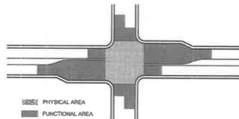
Figure 62. Comparison of physical and functional areas of an intersection. (87)
