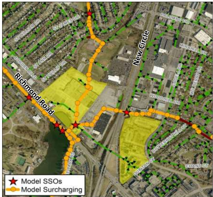
Figure 5.7. Sewer surcharging and SSOs predicted by the hydraulic model
