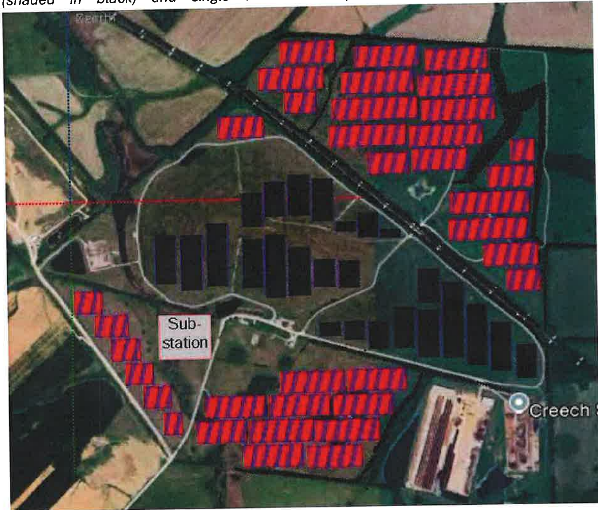
Image 2: Photovoltaic panel layout developed in PVSyst. Layout includes both fixed tilt (shaded in black) and single axis tracker panel sections (shaded in red).
