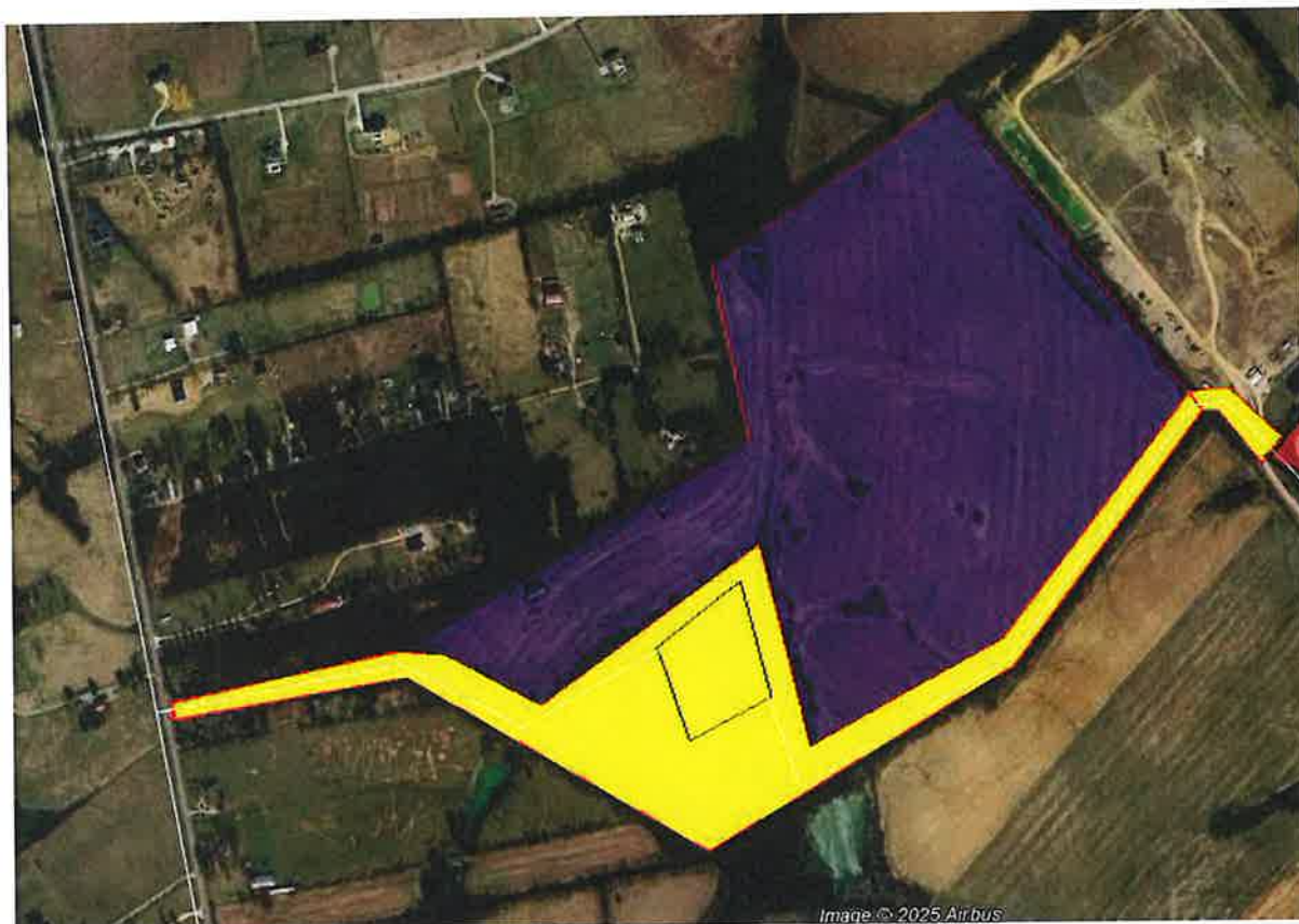
Image 5: Right of Way to utility point of connection line (shaded in yellow); the box outline represents the Switchyard to be constructed (i.e., marker #3 depicted in Image 1).
