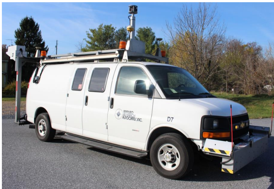
Figure 1. LCMS-based DSV with 360-degree ROW camera.
