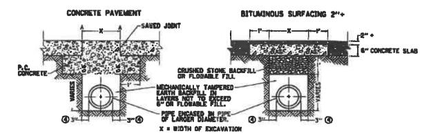
REPLACE CONCRETE PAVEMENT WITH NEW PAVEMENT SAME THICKNESS OF EXISTING PAVEMENT. REPAYE BITUMINOUS PAYEMENT STIN THE SAME TYPE MO BEPTH AS EXISTING PAYEMENT,
