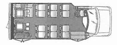
3.2 Seating: Unit shall have seating for twelve (12) passengers, one (1) driver, and two (2) wheelchairs. Two (2) fold away jump seats shall be provided in the wheelchair area for use by ambulatory passengers in the absence of wheelchair passengers. Jump seat mounting shall maintain as much clear path to rear emergency exit as practicable. All seats shall be high back, premium (level 4) vinyl upholstery, and provided with retractable seat belts and
