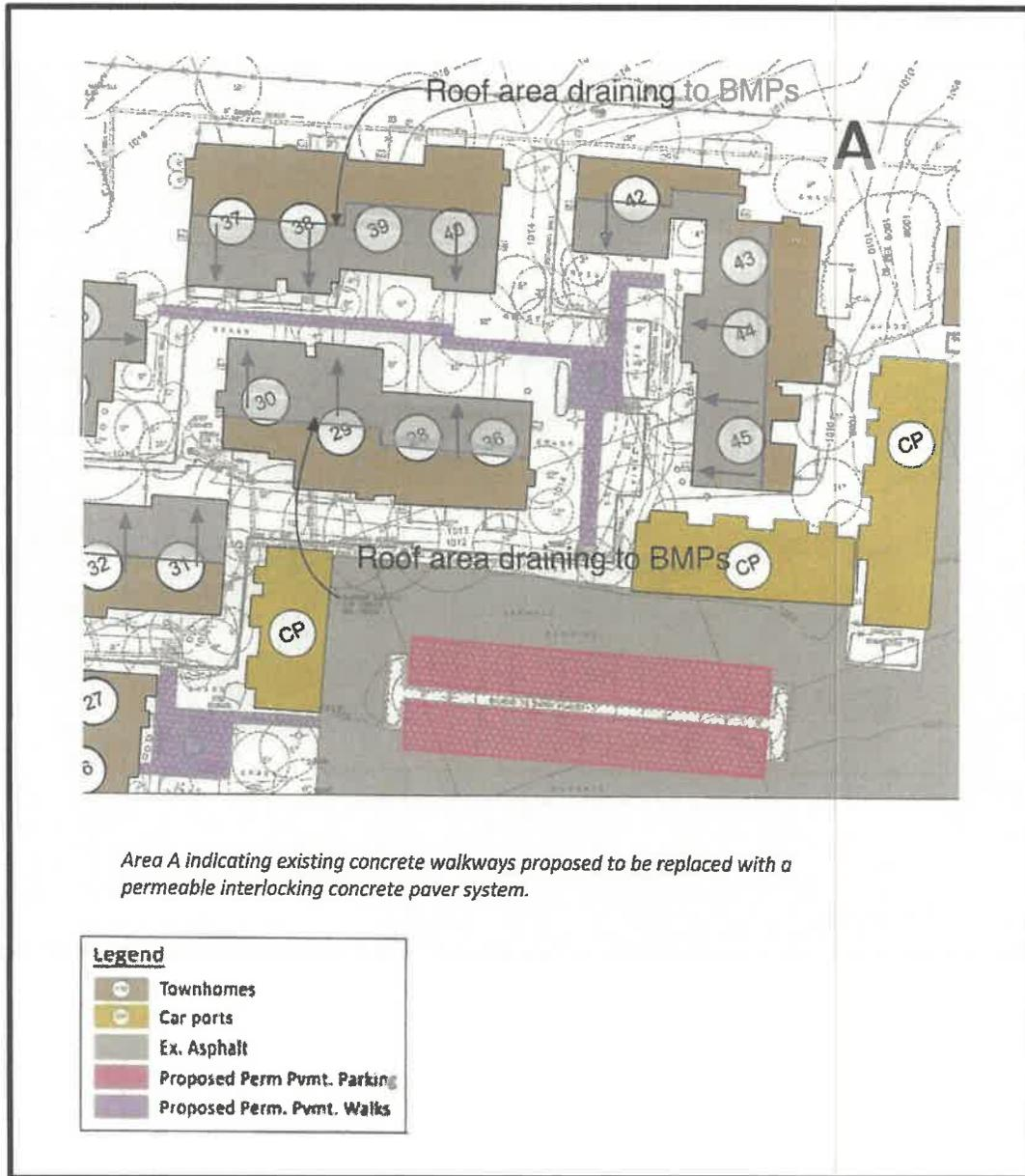
*Area A indicating existing concrete walkways proposed to be replaced with a permeable interlocking concrete paver system.*
