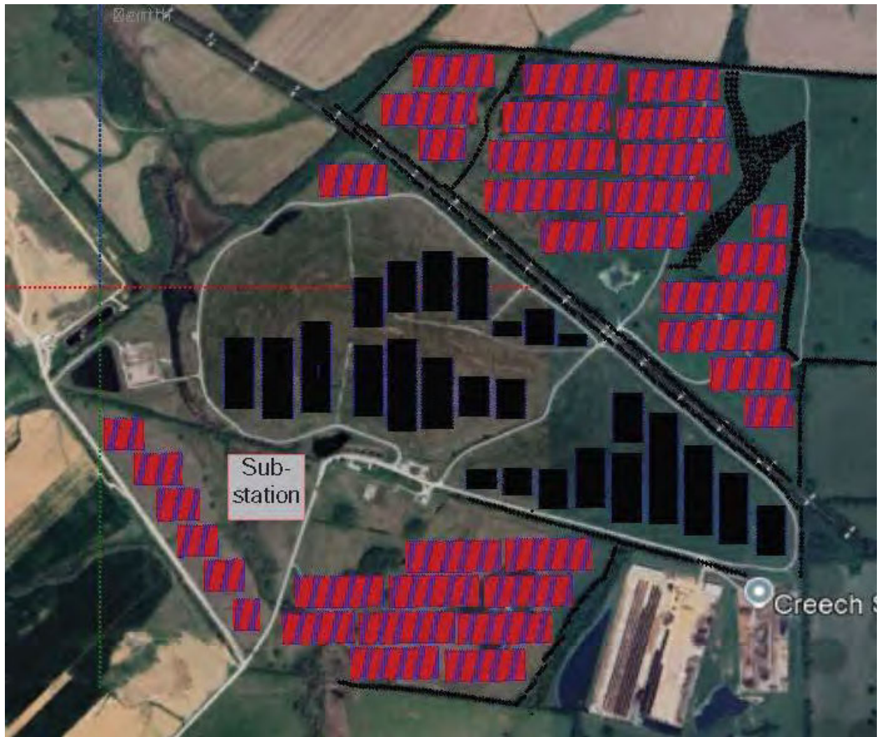
Image 2: Photovoltaic panel layout developed in PVSyst. Layout includes both fixed tilt (shaded in black) and single axis tracker panel sections (shaded in red).
