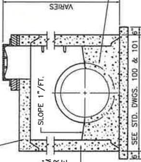
FOR CIRCULAR MANHOLE, WALLS SHALL MEET ASTM C-478 OR C-76. (FOR NON-CIRCULAR MANHOLE SEE STD. DWGS. 108, 110 & 113)
