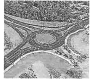
The multi-lane roundabout replaced a separated grade interchange at US 22 and SR 126 and opened in August 2021.
