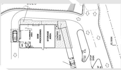
to conduct HHW collection events or to build a permanent site under various operating conditions. It was determined to be feasible to construct a permanent HHW facility at the Buckman Road Recycling/Transfer Station. JRMA completed design of a 3,000 sq ft block building that includes a storage area and a loading dock. JRMA also assisted the SFSWMA with developing an operational plan and prepared an RFP to select a TSD operator.
