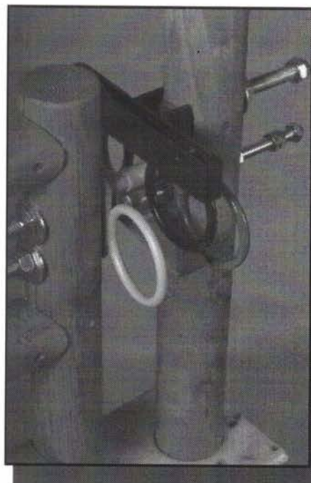
Figure 3—An Accessible Ring Latch with guard rings (gray and red) on both sides of the lever to make it difficult for horses to open the latch.
