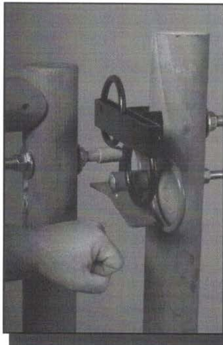
Figure 7—When the lever (green) is released, the gate begins to open.
