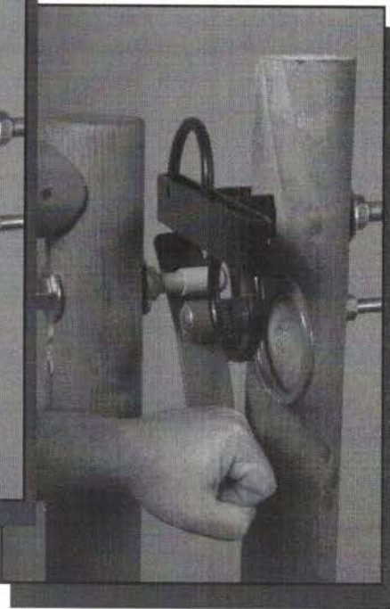
Figure 6—Pressure is applied to the gate and lever (green) at the same time, opening the gate.
