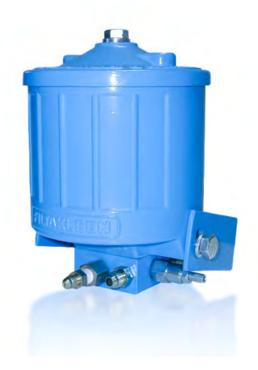
Filtakleen Bypass Hydraulic Oil Filters permanently maintain hydraulic oil at ISO 14/11 H20=<0.05%. The Filtakleen system can be either installed directly onto the machine or used as an off-line cleaning rig to purify the oil. The benefits to the oil and machine are two-fold: Ultra-fine Debris removal down to 1 micron which, is generally missed by the primary 10-micron filter.
