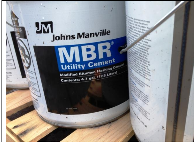
Photograph #1: Roof Flashing Cement
