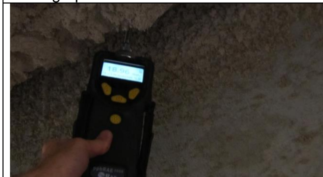
Photograph #7: High PID at drip (19 ppm)
