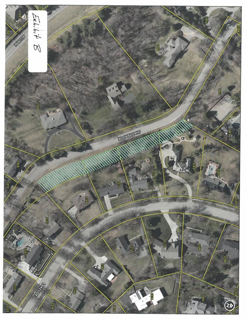
The 40' of right of way was dedicated in 1966 per the referenced plat to allow for the relocation of this section of Mt. Tabor Road now known as Shadybrook Lane. It appears the road was not relocated per the final record plat and this would explain the deed discrepancy with the GIS information per the exhibits provided.
