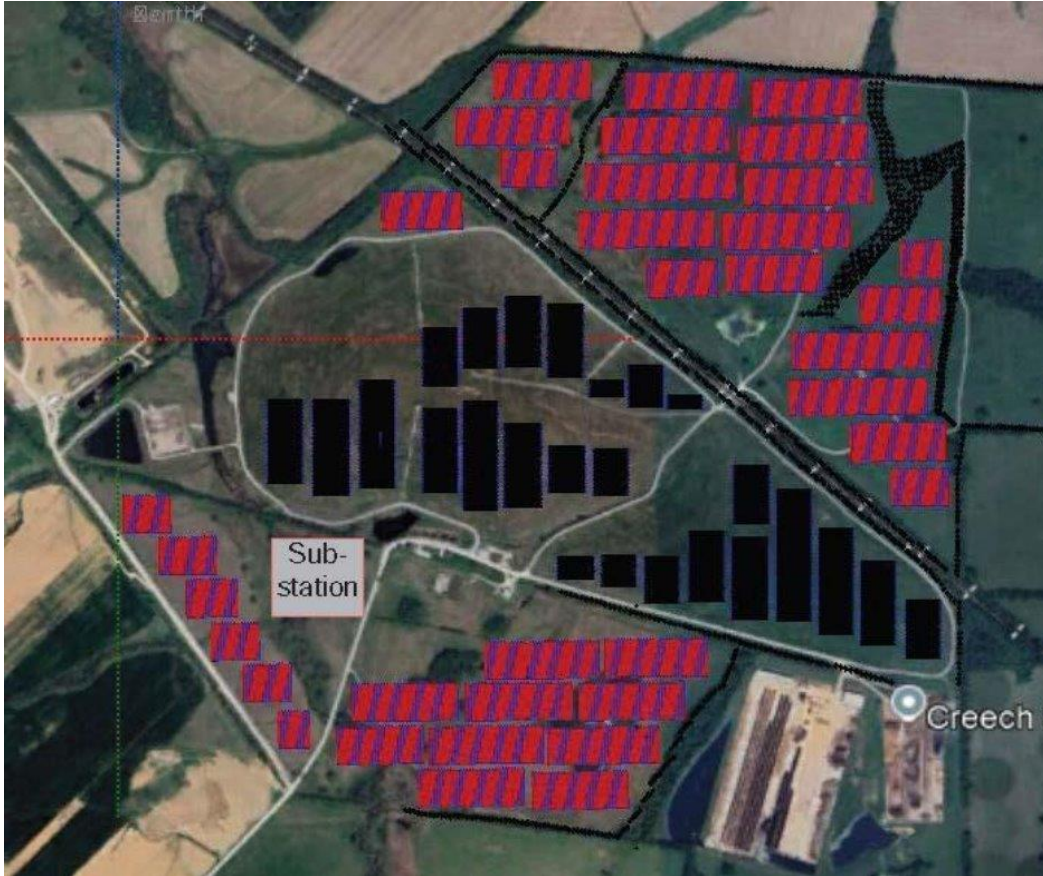
Proposed HPSP layout; includes both fixed tilt (black) and single axis tracker panel sections (red).
