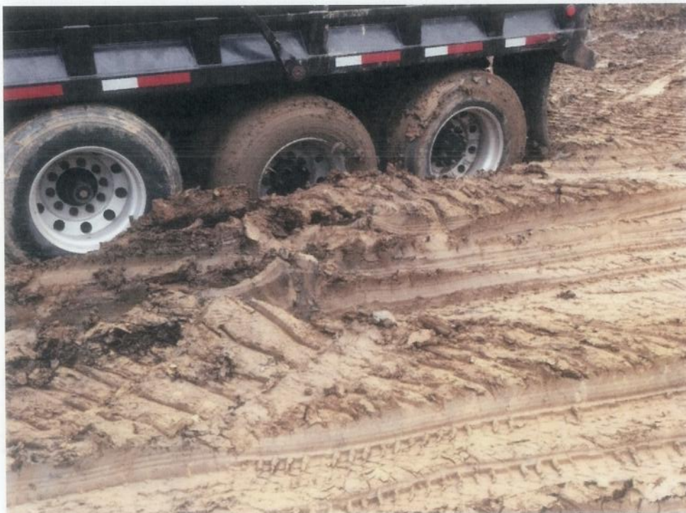
Photo 4: View Of Truck Rutting During The Proof Roll
