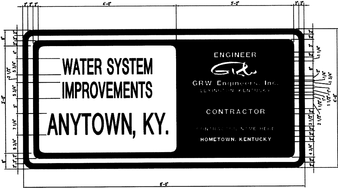
Figure 1: Typical Project Sign
