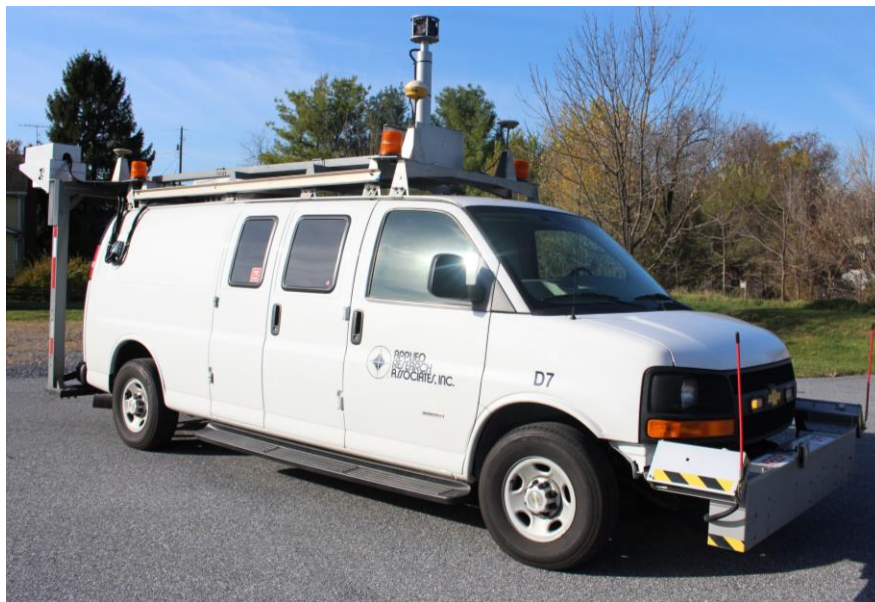
Figure 1. LCMS-based DSV with 360-degree ROW camera.
