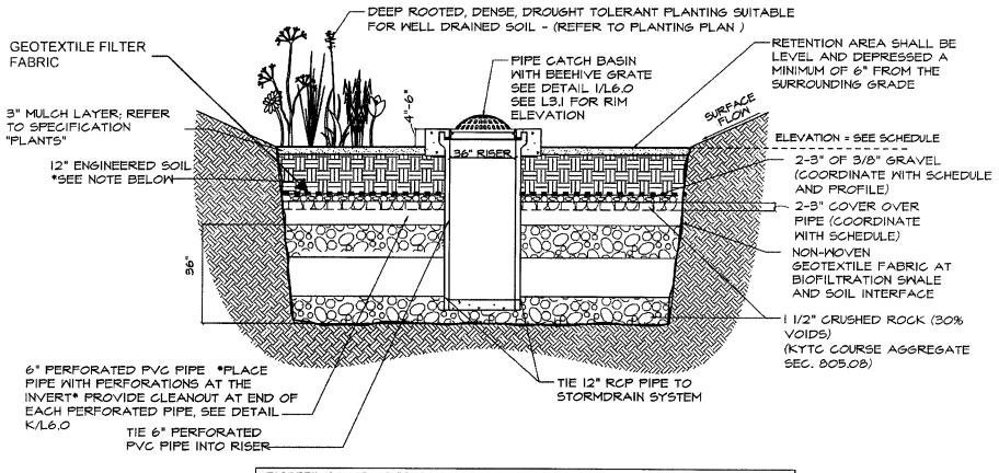
\*BIORETENTION "ENGINEERED SOIL" LAYER SHALL BE "SANDY LOAM" SOIL MIX WITH NO MORE THAN 5% CLAY CONTENT. THE MIX SHALL CONTAIN 50-60% SAND, 20-30% COMPOST OR HARDWOOD MULCH, AND 20-30% TOPSOIL.
