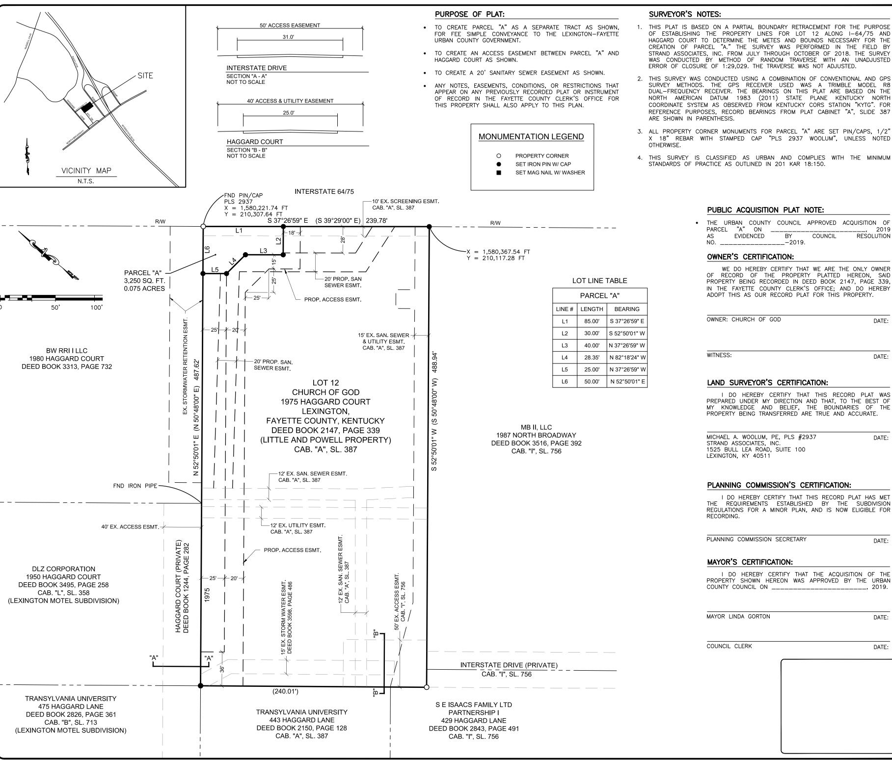
1. THIS PLAT IS BASED ON A PARTIAL BOUNDARY RETRACEMENT FOR THE PURPOSE OF ESTABLISHING THE PROPERTY LINES FOR LOT 12 ALONG I-64/75 AND HAGGARD COURT TO DETERMINE THE METES AND BOUNDS NECESSARY FOR THE CREATION OF PARCEL "A." THE SURVEY WAS PERFORMED IN THE FIELD BY STRAND ASSOCIATES, INC. FROM JULY THROUGH OCTOBER OF 2018. THE SURVEY WAS CONDUCTED BY METHOD OF RANDOM TRAVERSE WITH AN UNADJUSTED
