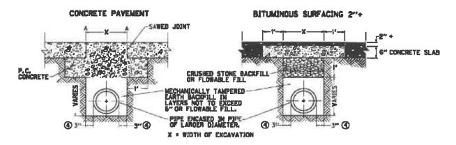
REPLACE CONCRETE PAYEMENT WITH NEW PAYEMENT SAME THICKNESS OF EXISTING PAYEMENT. REPAVE BITUNDHOUS PAYEMENT WITH THE SAME TYPE AND DEPTH AS EXISTING PAYEMENT.
